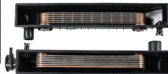
OSC: 7-Plate Stainless Steel Trans & 6-Plate Engine Oil Coolers
