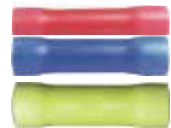
BUTT CONNECTORS VINYL INSULATED 1700CS - RED, 22-18 GA 1800CP - BLUE, 16-14 GA 1900CP - YELLOW, 12-10 GA
