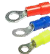
RING INSULATED CONNECTORS #10 - VINYL INSULATED 1705CS - RED, 22-18 GA 1805CS - BLUE, 16-14 GA 1905CP - YELLOW, 12-10 GA
