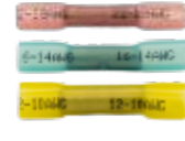
BUTT CONNECTORS VINYL INSULATED 1700CS - RED, 22-18 GA 1800CP - BLUE, 16-14 GA 1900CP - YELLOW, 12-10 GA
